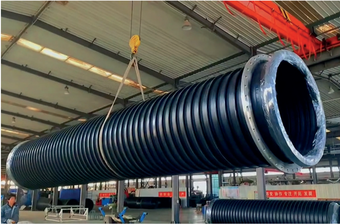
Spiral-wound reinforced PE pressure pipe at the Shunfang factory.
